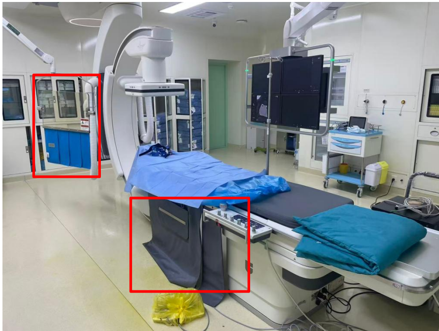
床下铅帘和悬吊铅帘
